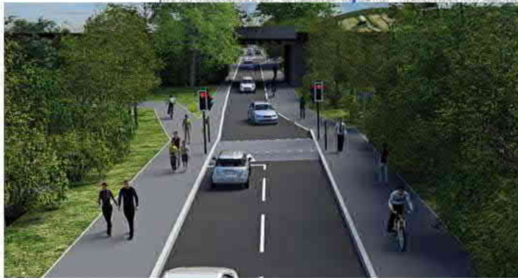
Visualisation of possible shared use footway/cycleway under the rail bridge on The Straight Mile, looking towards Hereford Enterprise Zone. Shows toucan crossing and the priority working for motor vehicles under rail bridge
